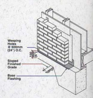
NOTE: The above flashing detail also applies to brick work above openings, such as windows and doors.
